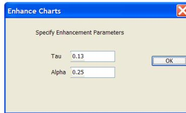
The parameters “Tau” and “Alpha” are selected to get the optimum inspection accuracy of the enhanced charts. Each sensor head has its own set of values. The values of “Tau” and “Alpha” shown are for an LMA-175 Sensor Head. Other Sensor Heads will have their own values.
